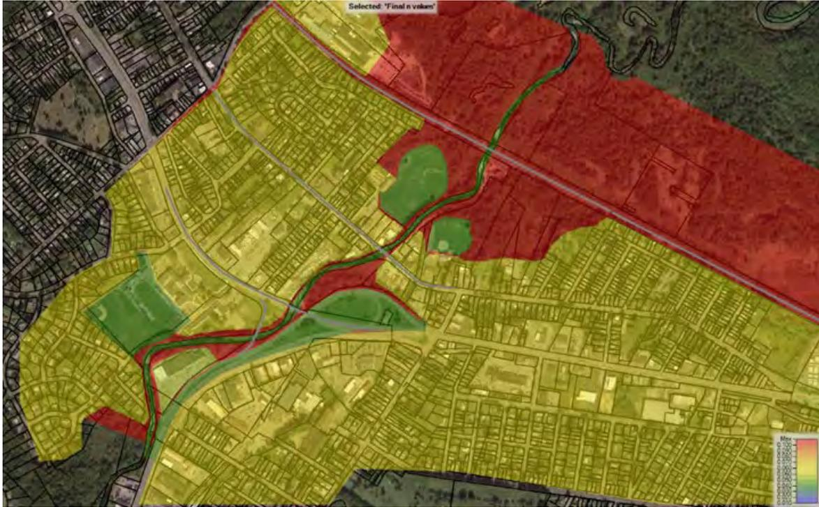
**Figure 2. Calibrated Manning's n for the 2d Model**
