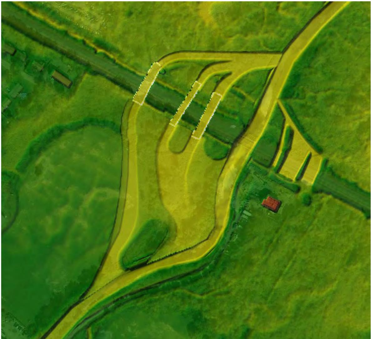
Figure 41. Proposed Flood Bench near the Railroad Crossing of Sauquoit Creek
