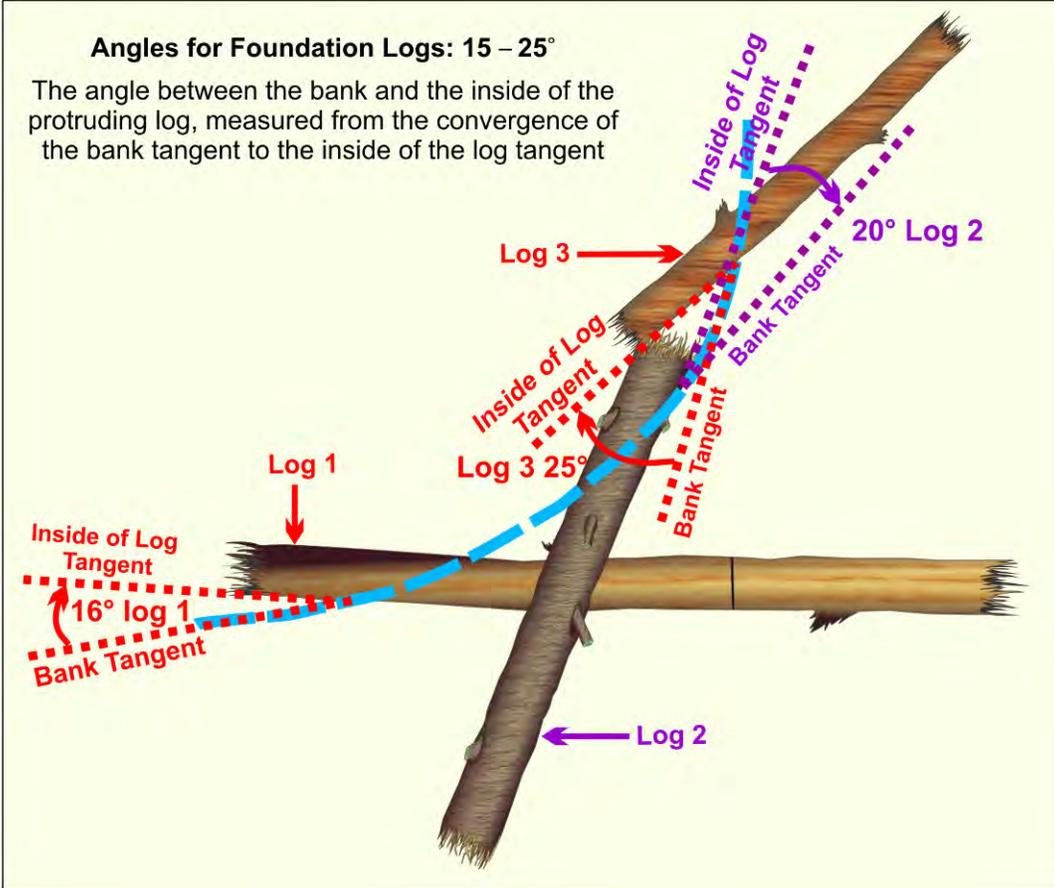
**Step 5.** Place root wad logs cantilevered over foundation logs
