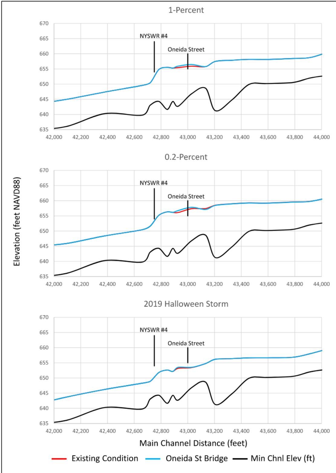
**Figure 5-22. (continued) HEC-RAS model output for the existing conditions (red) and proposed increase bridge span of the Oneida Street bridge (blue) scenarios.**
