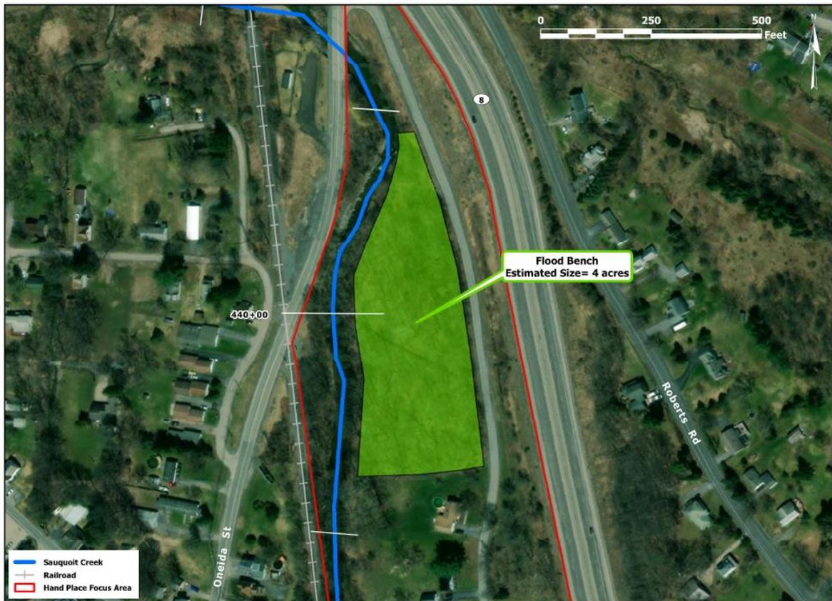
**Figure 5-16. Conceptual depiction of flood benches proposed for the Hand Place area.**
