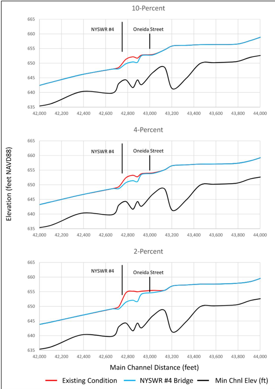
**Figure 5-14. (continued) HEC-RAS model output for the existing conditions (red) and proposed increased hydraulic capacity of NYSWR #4 bridge (blue) scenarios.**
