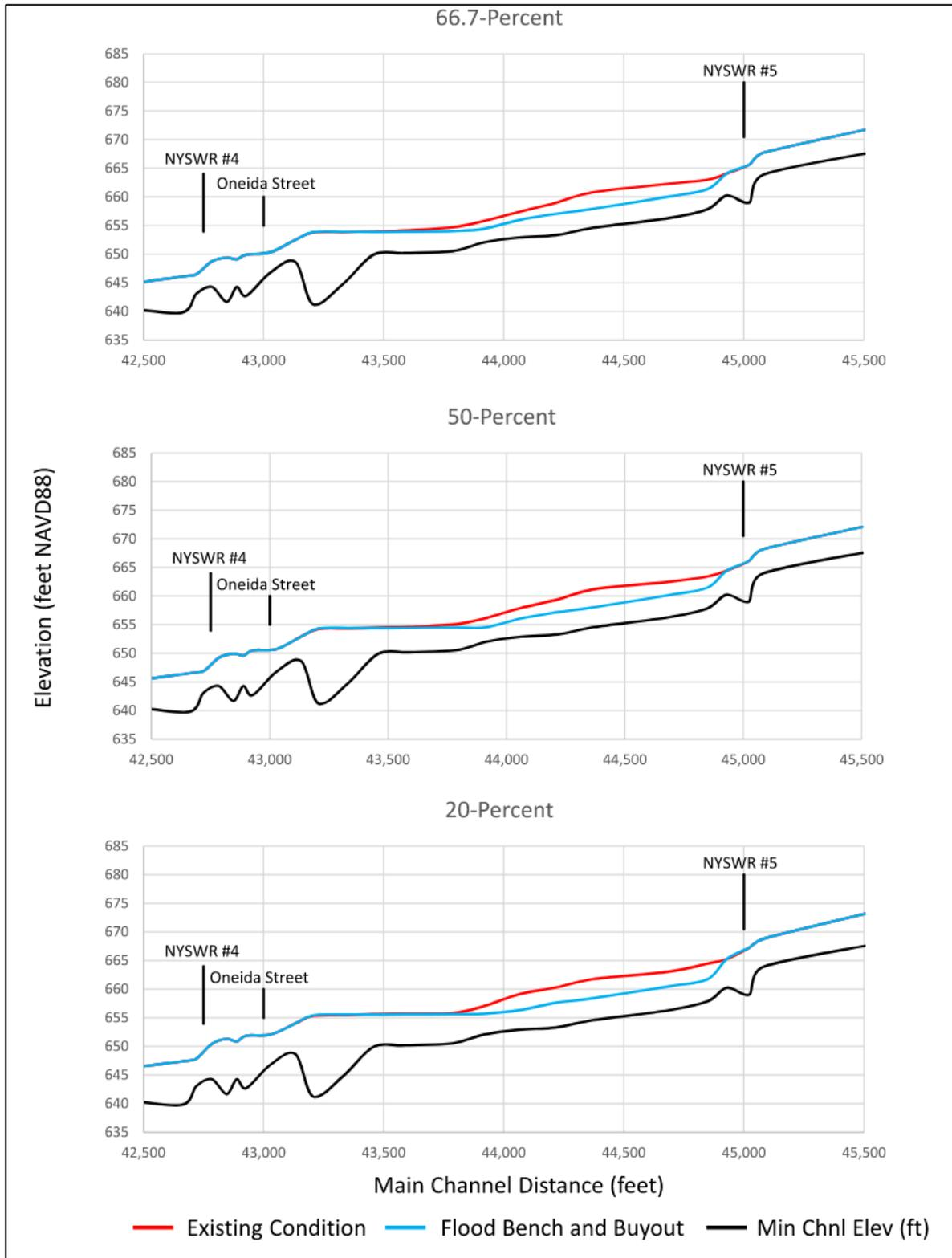
**Figure 5-19. HEC-RAS model output for the existing conditions (red) and proposed flood bench (blue) scenarios.**
