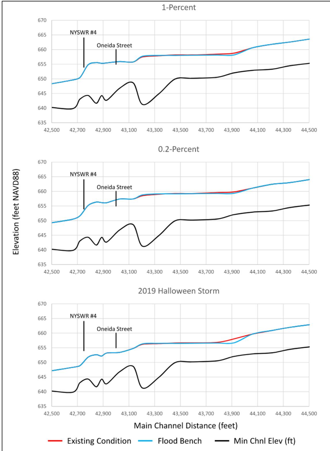
Figure 5-17. (continued) HEC-RAS model output for the existing conditions (red) and proposed flood bench (blue) scenarios.
