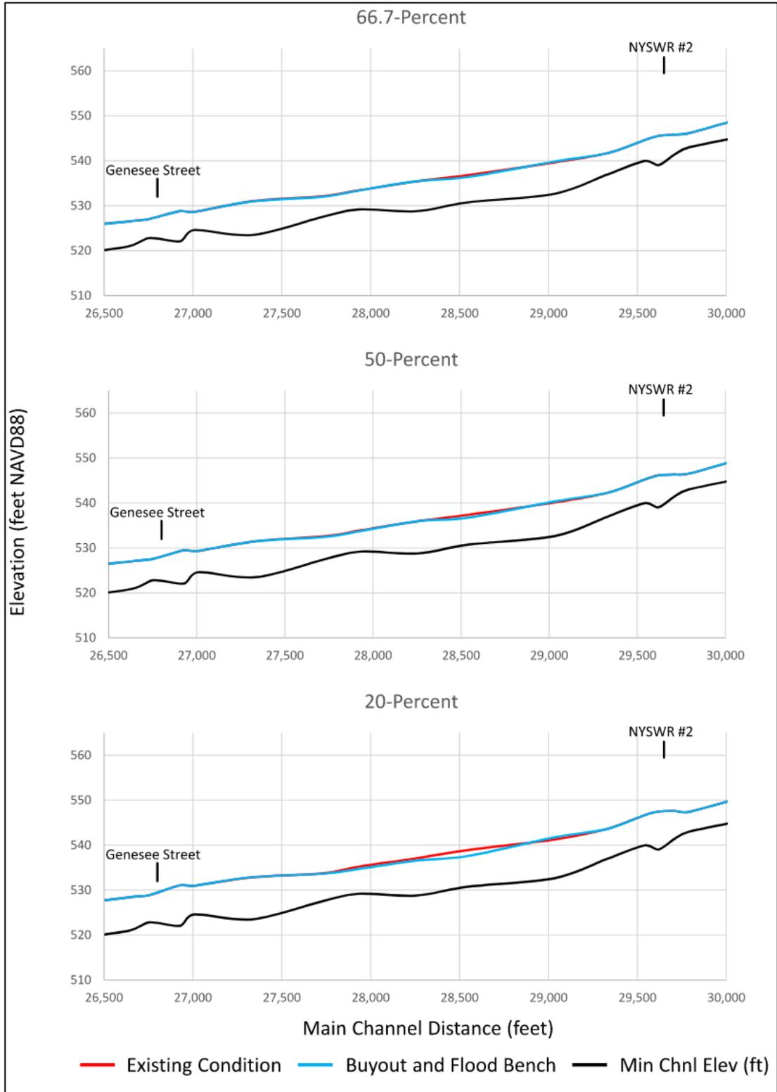
Figure 5-7. HEC-RAS model output for the existing conditions (red) and proposed buyout and flood bench (blue) scenarios.
