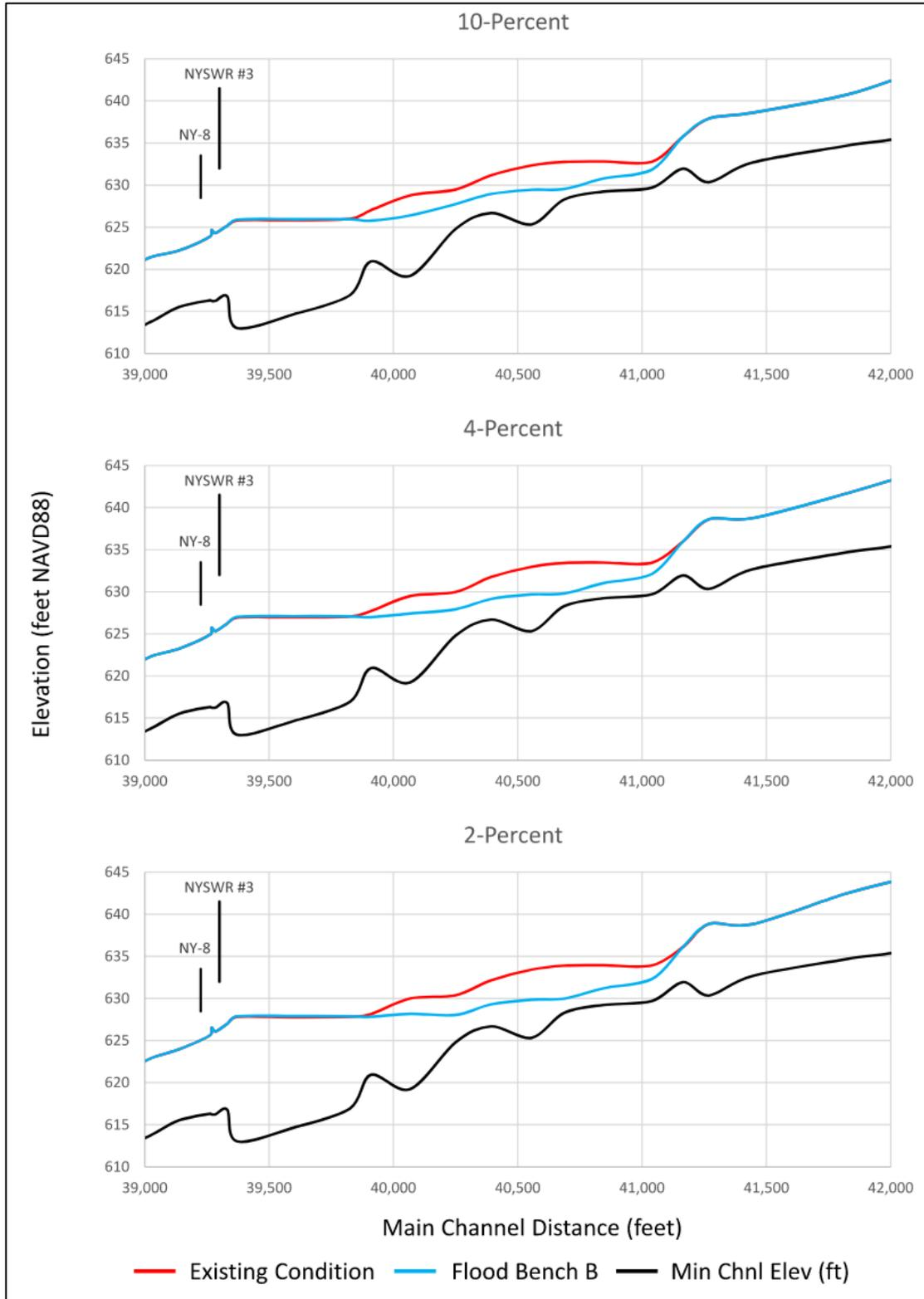
**Figure 5-11. (continued) HEC-RAS model output for the existing conditions (red) and proposed Flood Bench B (blue) scenarios.**
