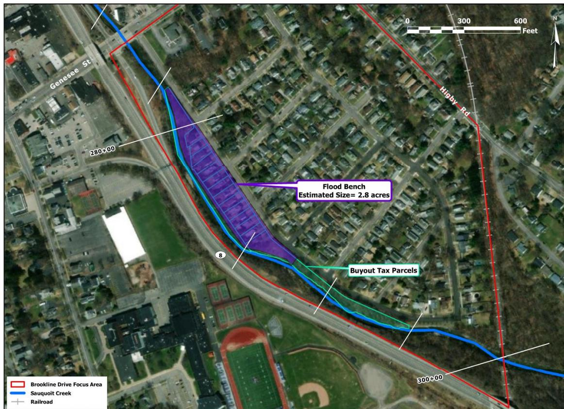
**Figure 5-6. Conceptual depiction of flood-prone property buyout and flood bench proposed for the Brookline Drive area.**
