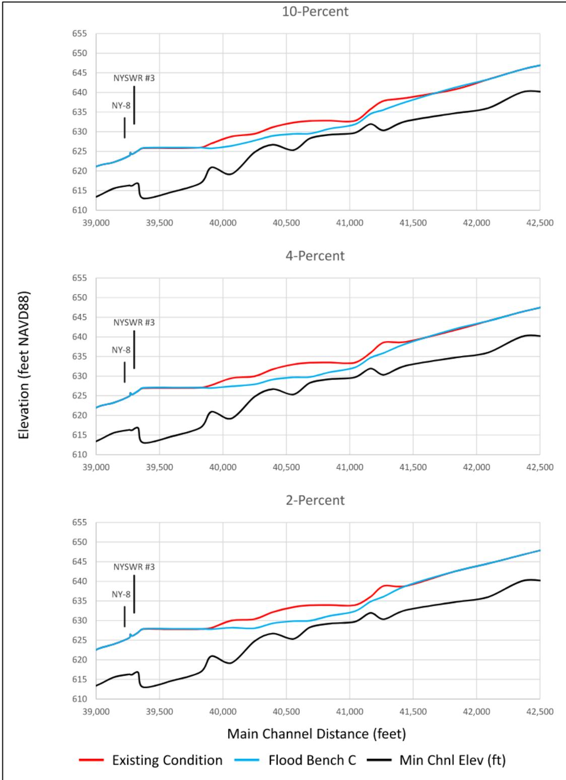
**Figure 5-12. (continued) HEC-RAS model output for the existing conditions (red) and proposed Flood Bench C (blue) scenarios.**
