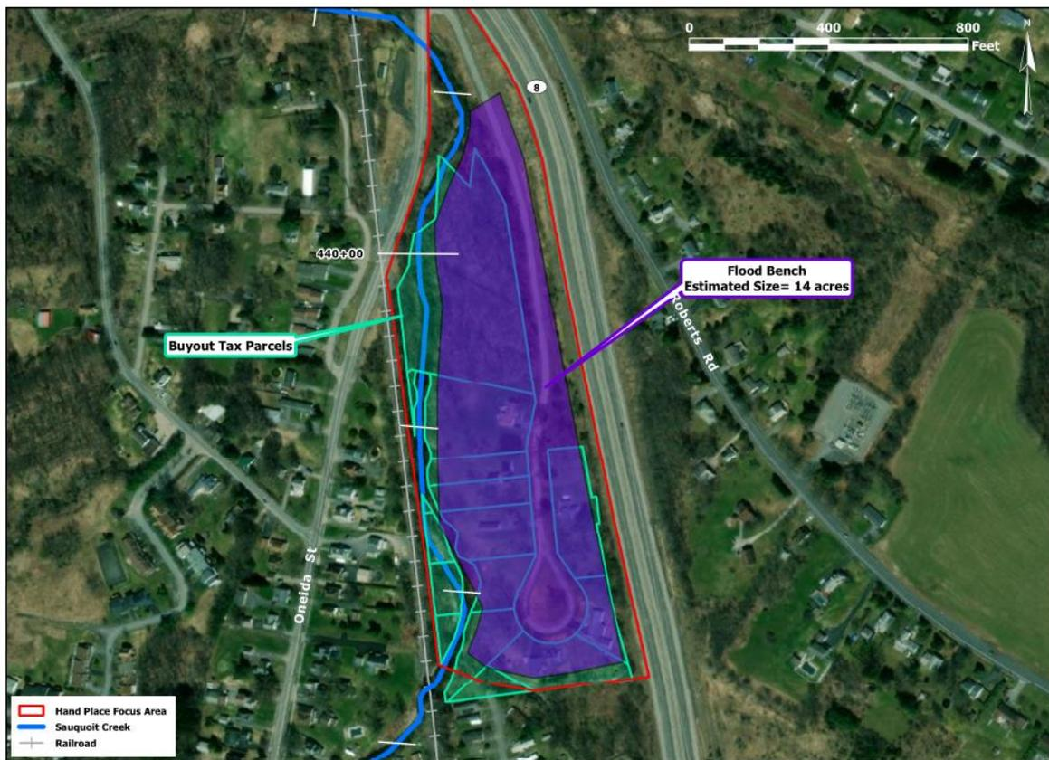
**Figure 5-18. Conceptual depiction of flood prone property buyout and flood bench proposed for the Hand Place area.**
