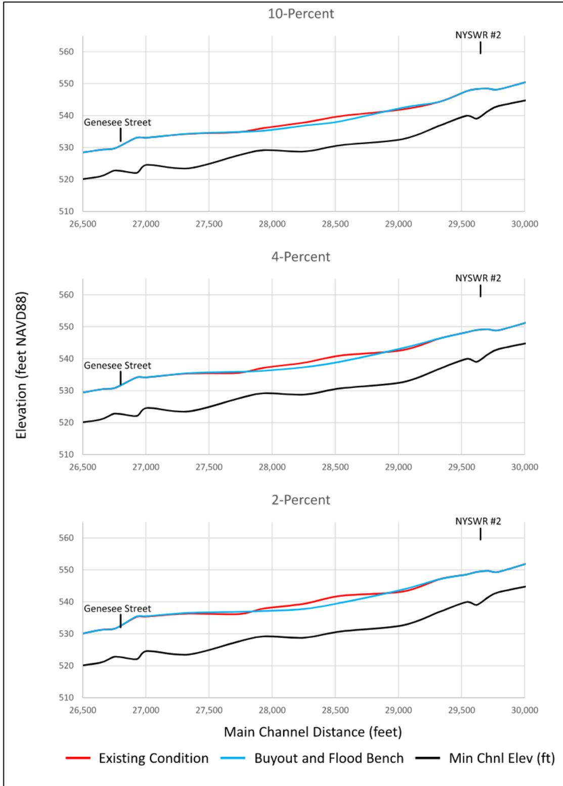
**Figure 5-7. (continued) HEC-RAS model output for the existing conditions (red) and proposed buyout and flood bench (blue) scenarios.**
