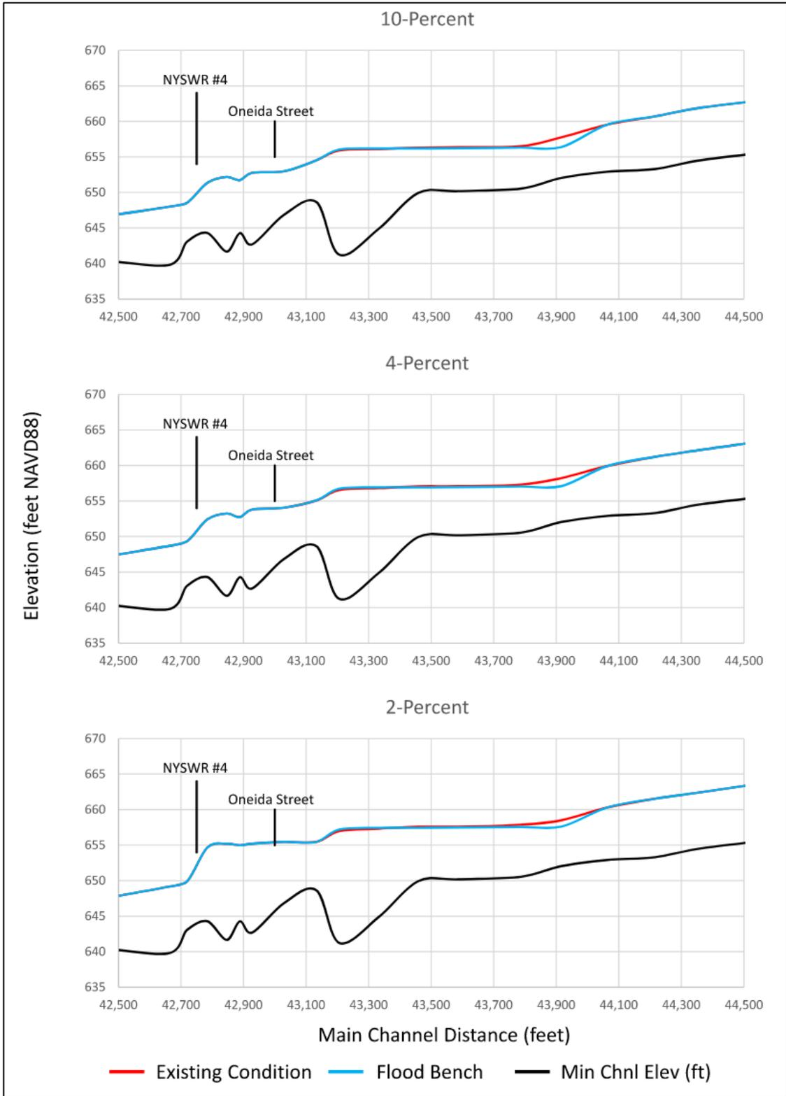
Figure 5-17. (continued) HEC-RAS model output for the existing conditions (red) and proposed flood bench (blue) scenarios.
