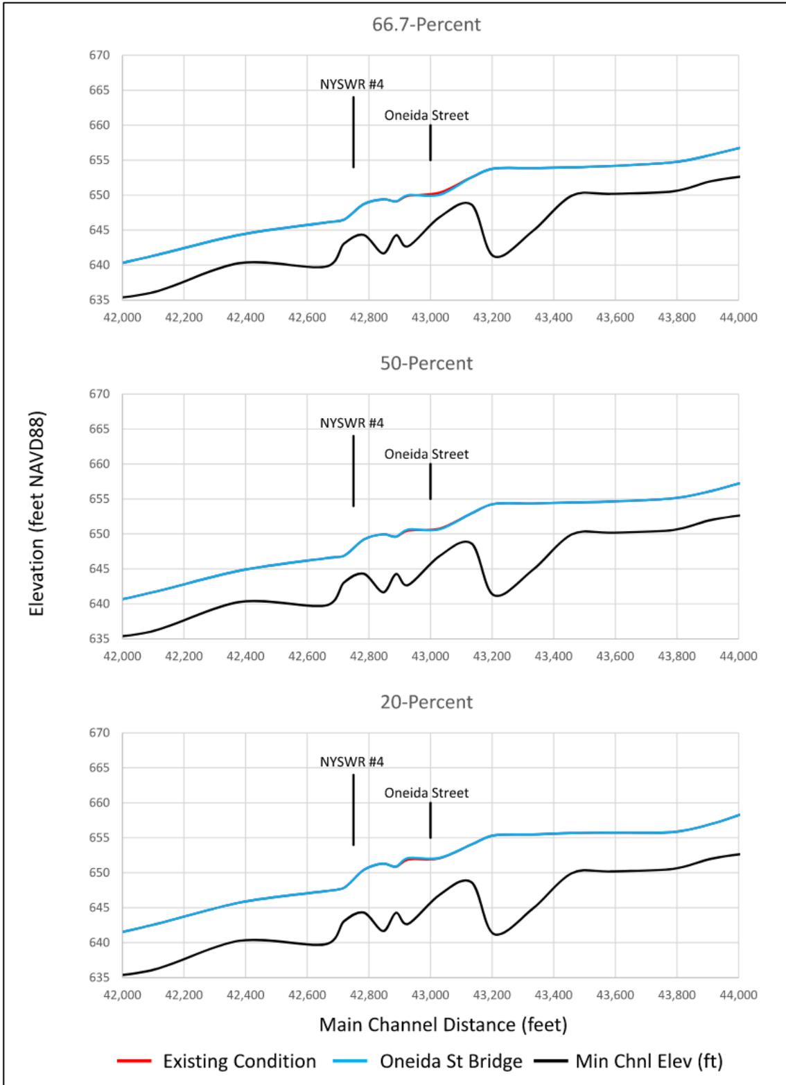
**Figure 5-22. HEC-RAS model output for the existing conditions (red) and proposed increase bridge span of the Oneida Street bridge (blue) scenarios.**
