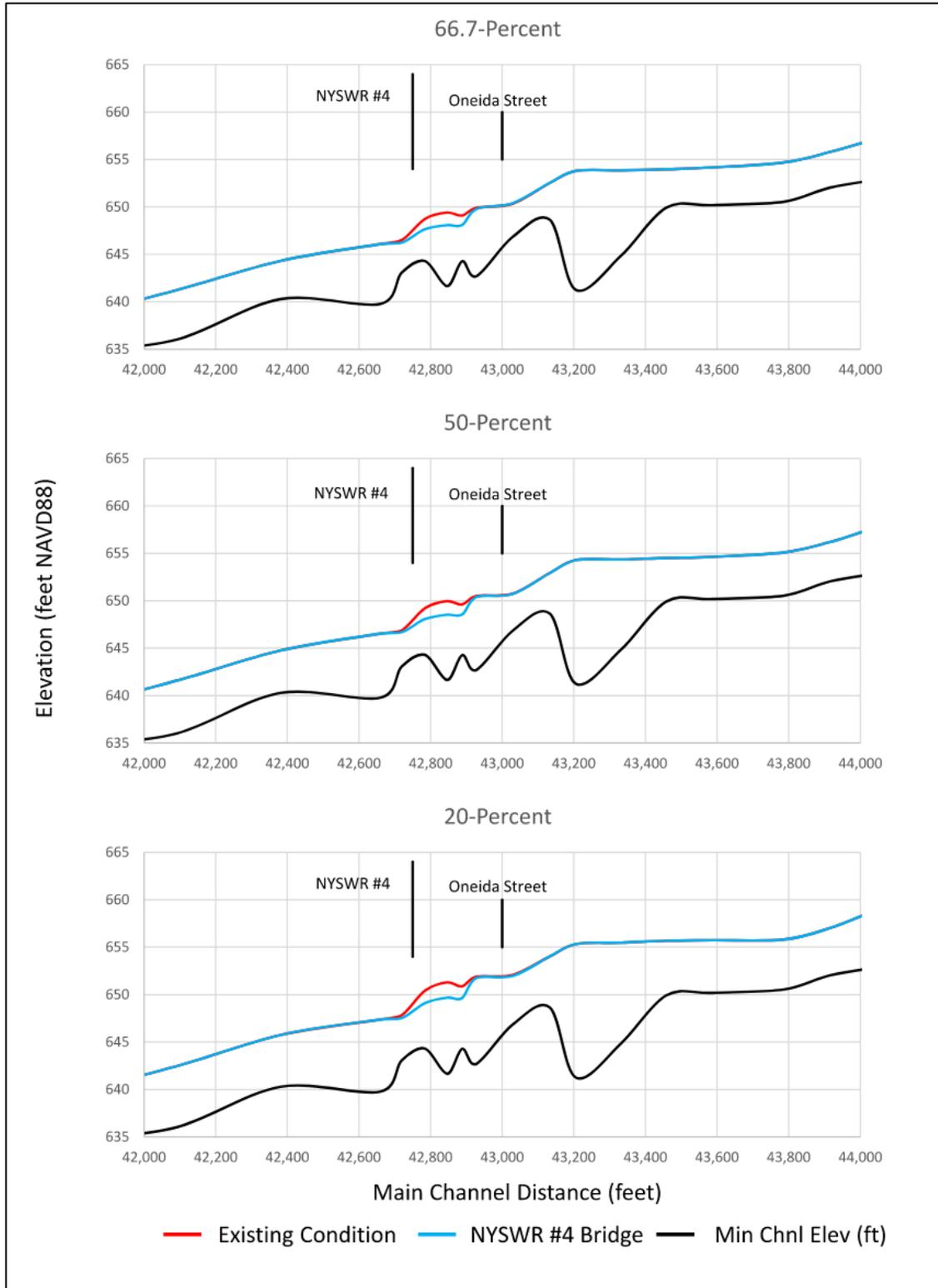
**Figure 5-14. HEC-RAS model output for the existing conditions (red) and proposed increased hydraulic capacity of NYSWR #4 bridge (blue) scenarios.**
