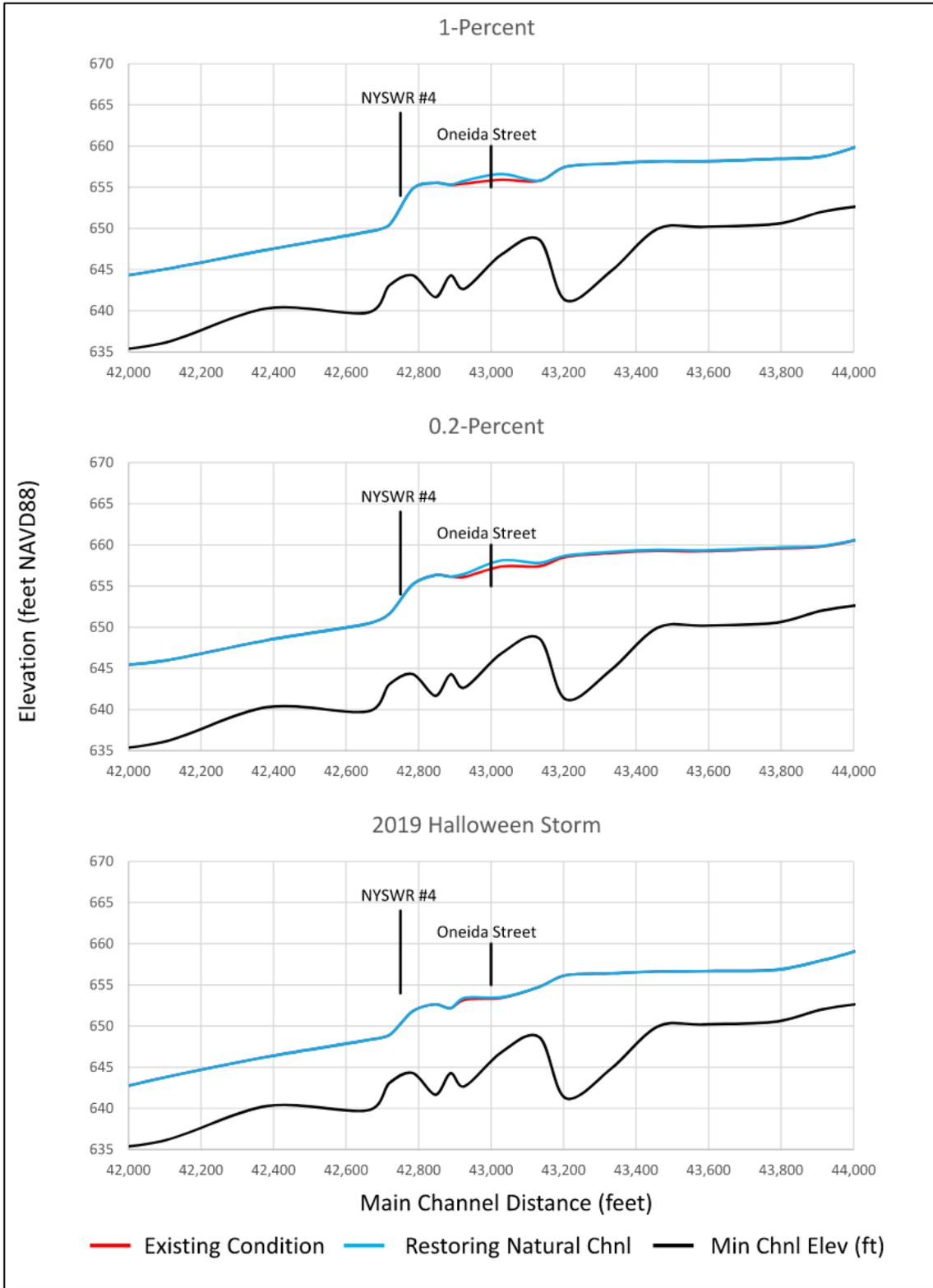
**Figure 5-21. (continued) HEC-RAS model output for the existing conditions (red) and proposed restoring natural channel geomorphology of the Oneida Street bridge (blue) scenarios.**
