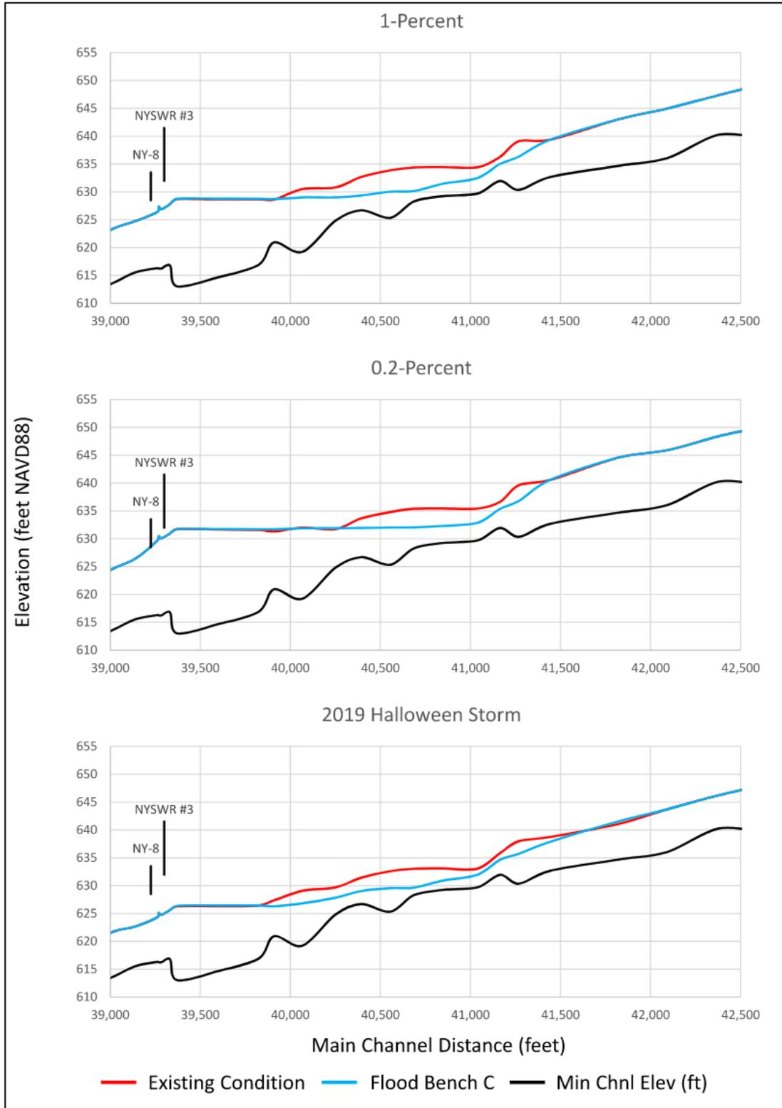
Figure 5-12. (continued) HEC-RAS model output for the existing conditions (red) and proposed Flood Bench C (blue) scenarios.
