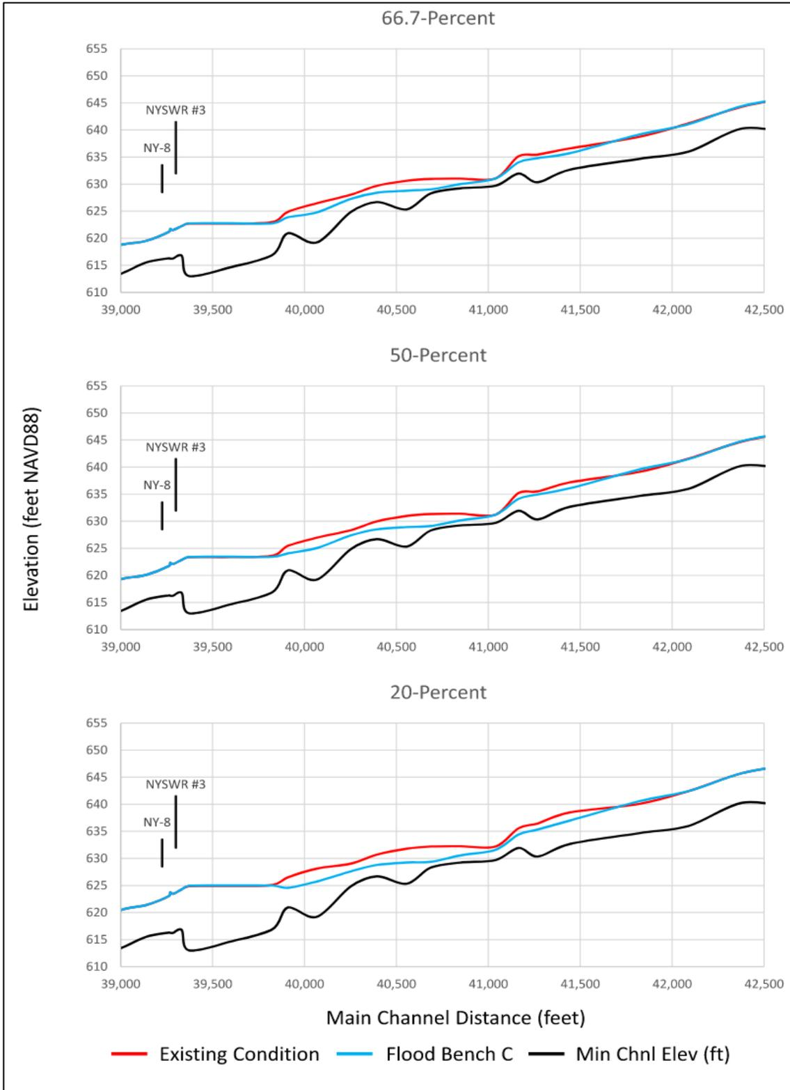
**Figure 5-12. HEC-RAS model output for the existing conditions (red) and proposed Flood Bench C (blue) scenarios.**
