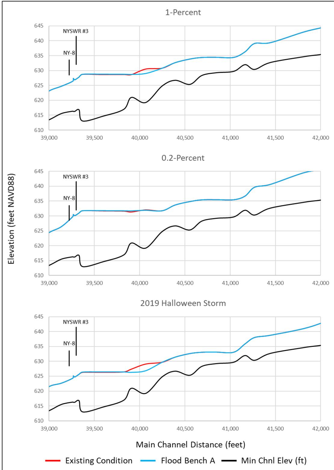
**Figure 5-10. (continued) HEC-RAS model output for the existing conditions (red) and proposed Flood Bench A (blue) scenarios.**
