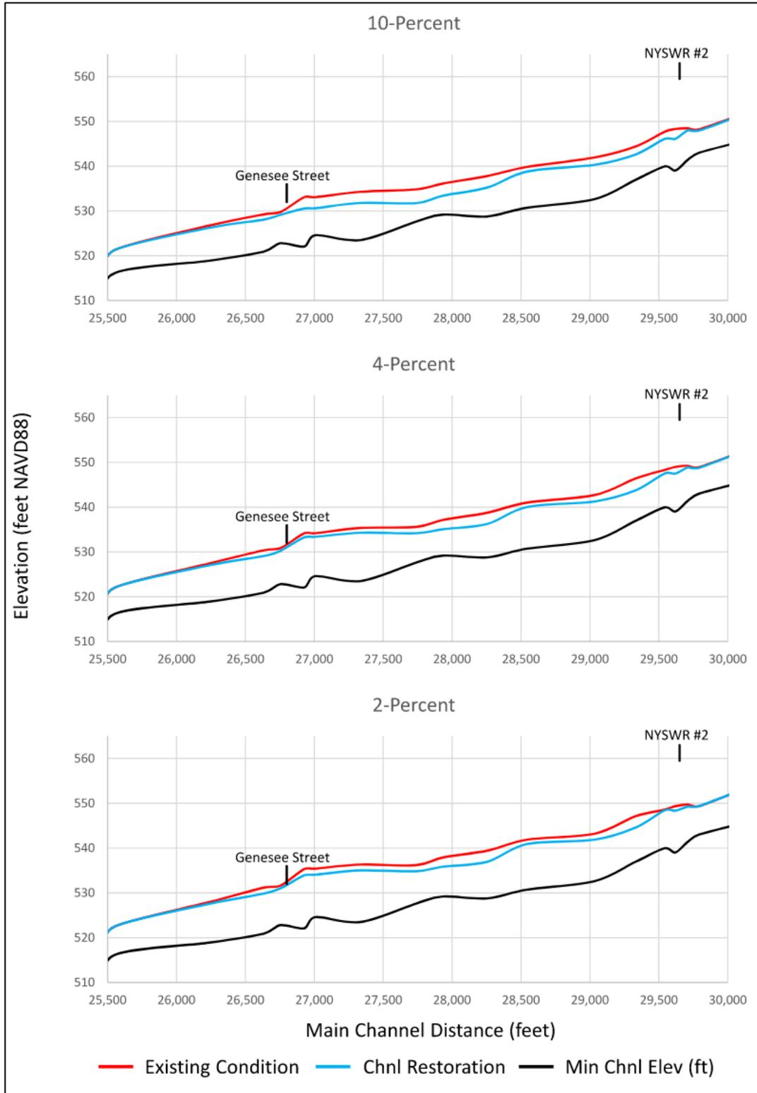
**Figure 5-4. (continued) HEC-RAS model output for the existing conditions (red) and proposed stream and channel restoration (blue) scenarios.**
