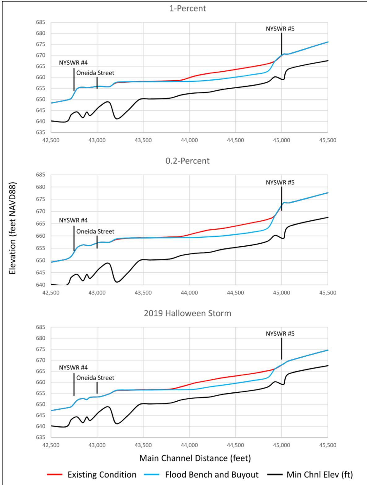
Figure 5-19. (continued) HEC-RAS model output for the existing conditions (red) and proposed flood bench (blue) scenarios.
