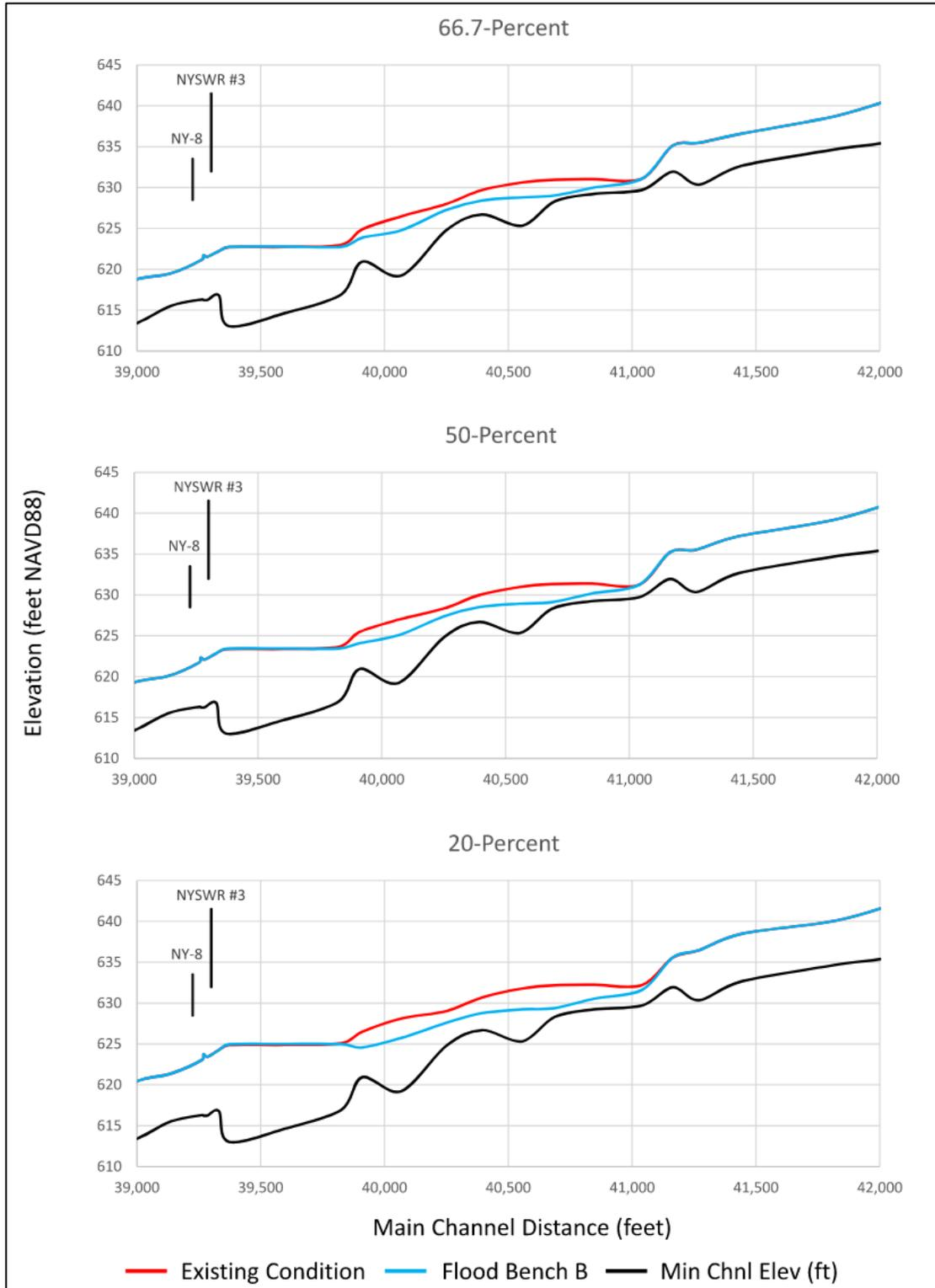
**Figure 5-11. HEC-RAS model output for the existing conditions (red) and proposed Flood Bench B (blue) scenarios.**
