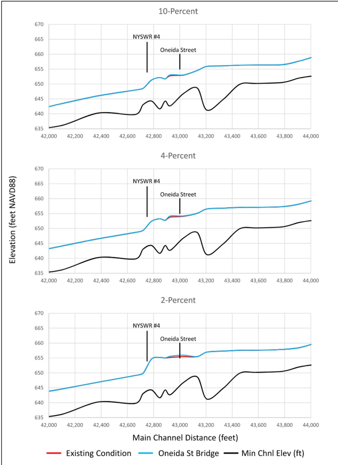
**Figure 5-22. (continued) HEC-RAS model output for the existing conditions (red) and proposed increase bridge span of the Oneida Street bridge (blue) scenarios.**
