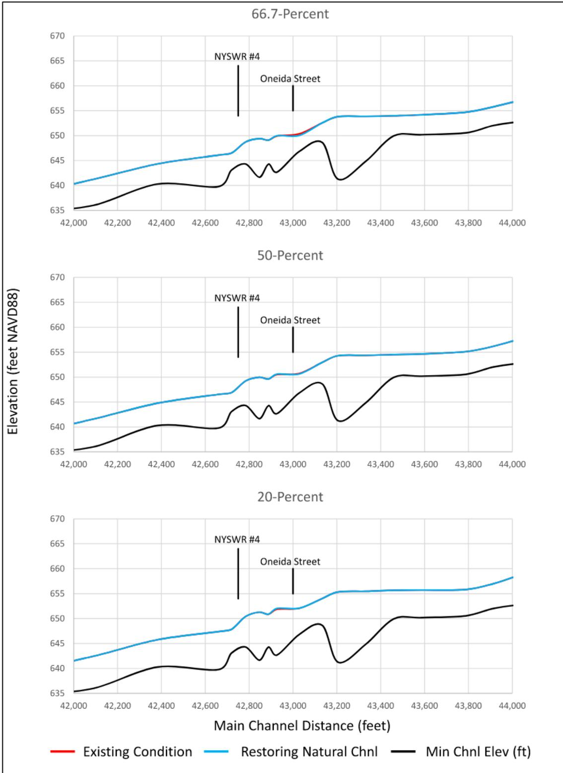
**Figure 5-21. HEC-RAS model output for the existing conditions (red) and proposed restoring natural channel geomorphology of the Oneida Street bridge (blue) scenarios.**
