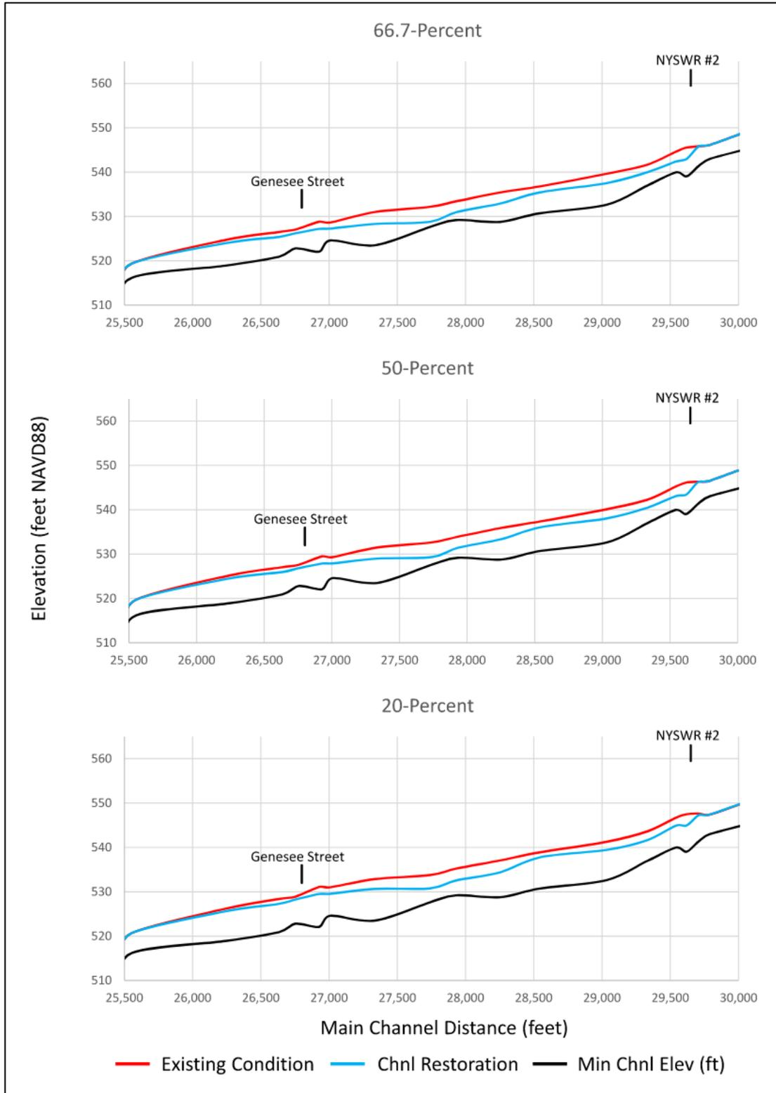
Figure 5-4. HEC-RAS model output for the existing conditions (red) and proposed stream and channel restoration (blue) scenarios.
