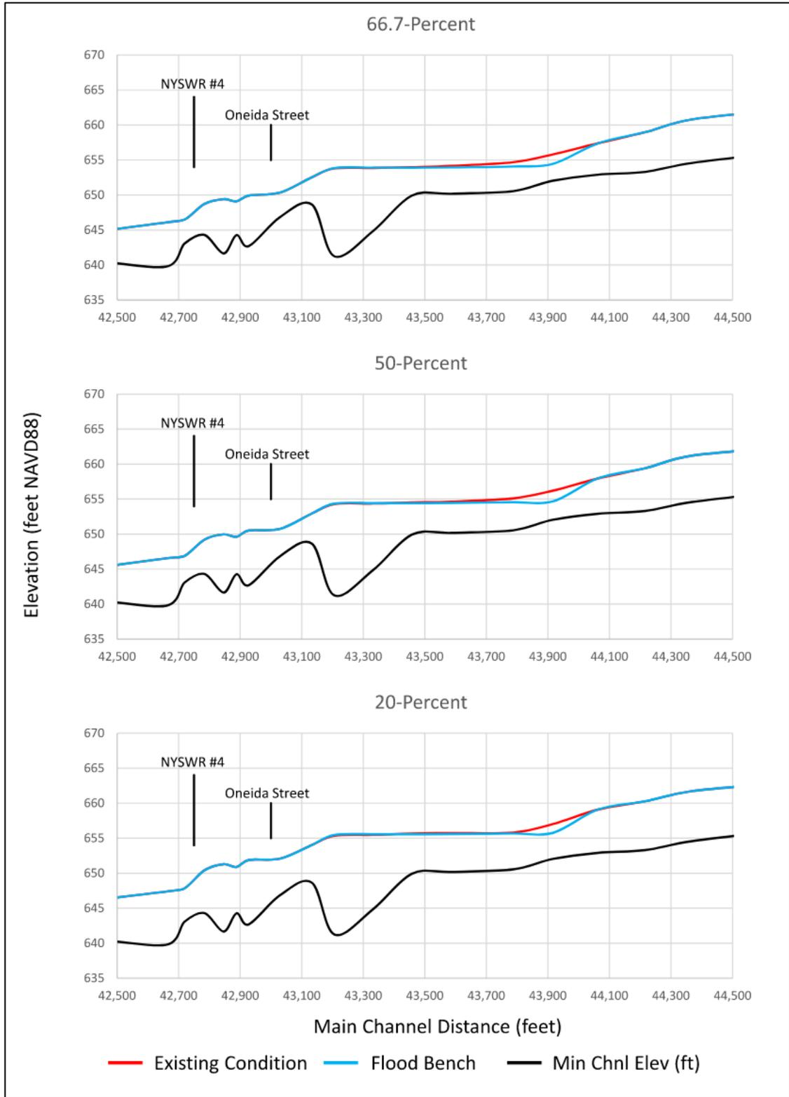
Figure 5-17. HEC-RAS model output for the existing conditions (red) and proposed flood bench (blue) scenarios.
