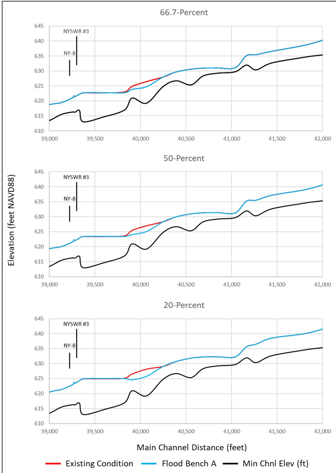
**Figure 5-10. HEC-RAS model output for the existing conditions (red) and proposed Flood Bench A (blue) scenarios.**
