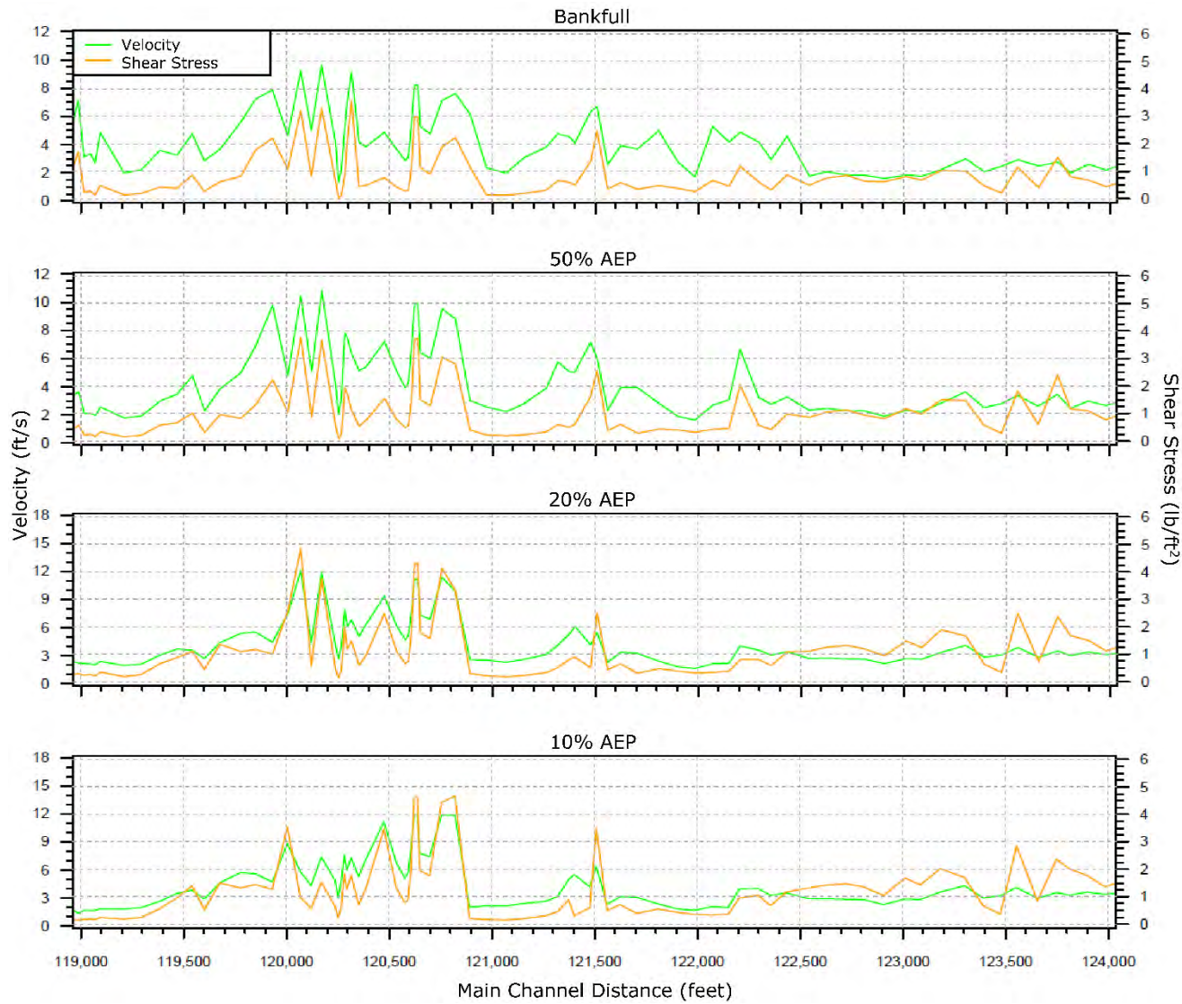
Figure 8-14. Analysis of velocity (ft/s) and shear stress (lbs/sq ft) based on the HEC-RAS model results for Zone 2.
