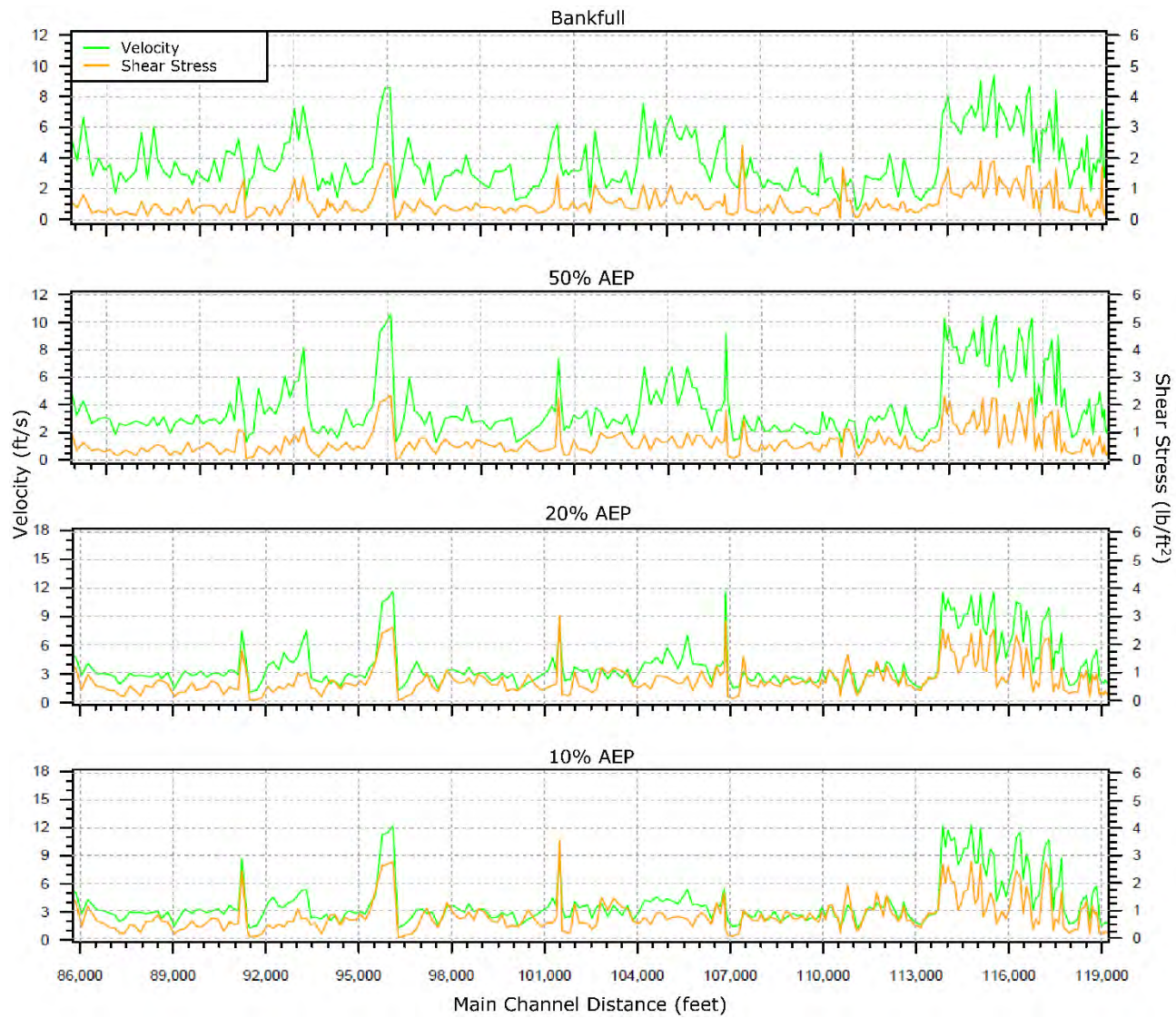
Figure 8-20. Analysis of velocity (ft/s) and shear stress (lbs./sq ft) based on the HEC-RAS model results for Zone 3.
