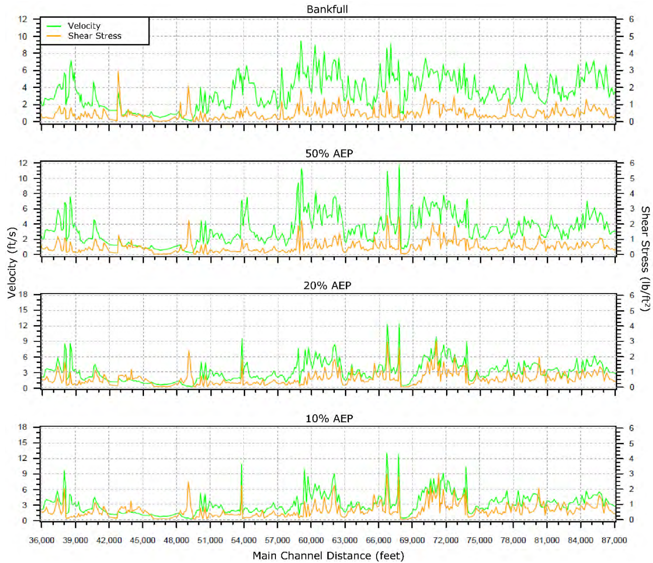
Figure 8-31. Analysis of velocity (ft/s) and shear stress (lbs./sq ft) based on the HEC-RAS model results for Zone 4.
