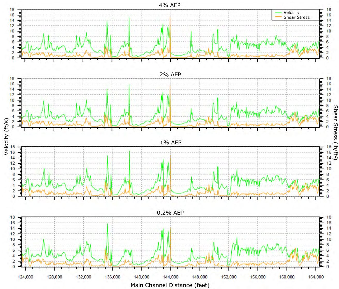
Figure 8-5 (continued). Analysis of velocity (ft/s) and shear stress (lbs/sq ft) based on the HEC-RAS model results for Zone 1.
