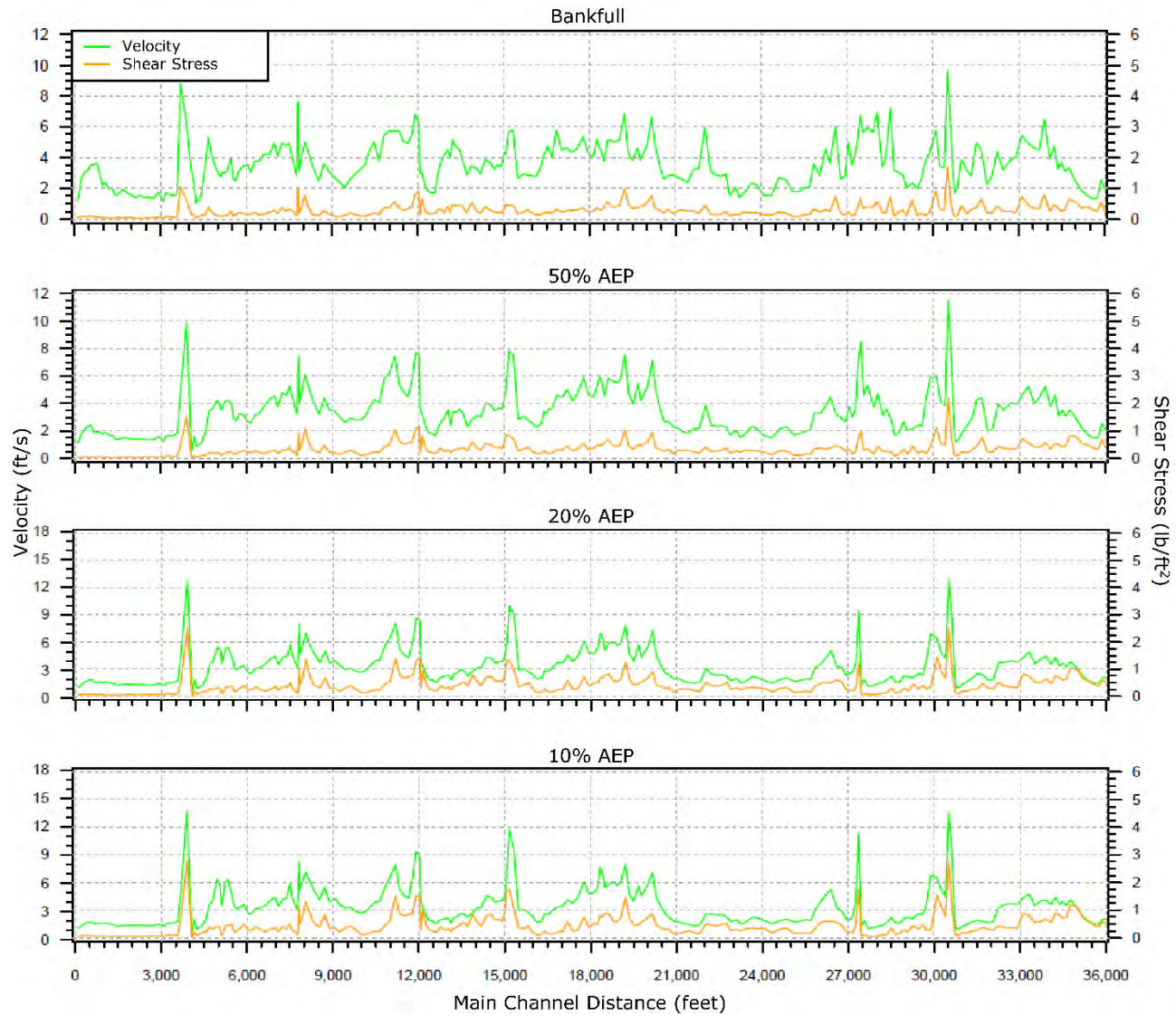
Figure 8-38. Analysis of velocity (ft/s) and shear stress (lbs./sq ft) based on the HEC-RAS model results for Zone 5.
